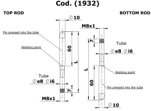
Since the rods must protrude by 17 mm. (see fig. 1 page 18), their length is calculated as follows:
