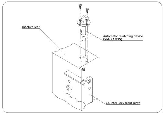
**Mounting diagram** This device is fitted at the top of the inactive leaf and fixed parallel to the door with two self-threading screws; use the two holes that allow tighter fastening.
