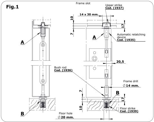
Insert the upper strike: with a click where it is possible or fix with the two self threading screws (in std. equip.). Insert the strike to the floor. Insert the rod bush: with a click where it is possible or fix with the two self threading screws (in std.equip.)
