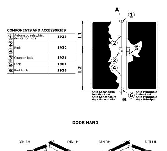
After the installation lubricate: the contact area between latchbolt and strike and between bottom pin rod and its strike.
