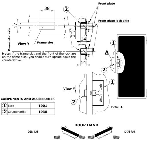
Insert the counterstrike in the frame slot with a click where it is possible or fix with the two self threading screws (in std.equip.). After the installation lubricate the contact area between latchbolt and strike.
