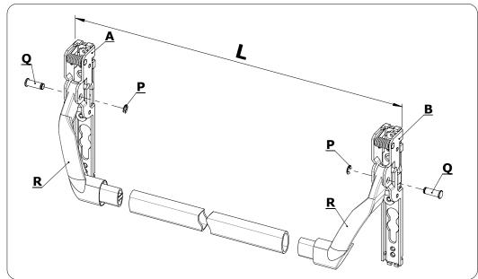
Measure the distance (L) between the two mechanisms (A) and (B). Cut the oval cross bar to a length equal to (L) minus **135 mm**. Press the oval cross bar into place in the side levers (**R**). The bar goes **18 mm**, into each lever.
