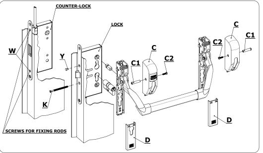
Make certain that all screws are completely tightened. Fix the bottom covers (D) first, then the top covers (C). Fix the top covers by fitting the screws (C1 e C2) into the two holes, lowering the two levers slightly.Where required, mount the cylinder (or single cylinder) and fix it with the screws ( $\mathbf{K}$ ). In the lock version insert the plastic plug ( $\mathbf{Y}$ ). Stop the upper and down rods with the proper screws ( $\mathbf{W}$ ) in the front holes of the counterlock.
