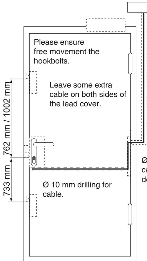
Please check the door gap if the lock case is surface mounted. The door gab should be min 8.5 mm and max 15 mm. (The gap between the strike and the lock case should be 2 - 5.5 mm.)
