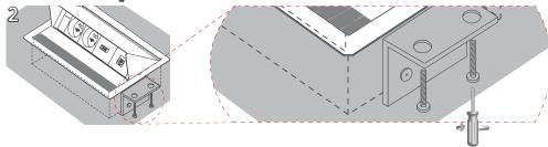
Assembling to the table top / desk of up to 30 mm thickness. Assembling to the table top / desk of up to 50 mm thickness.
