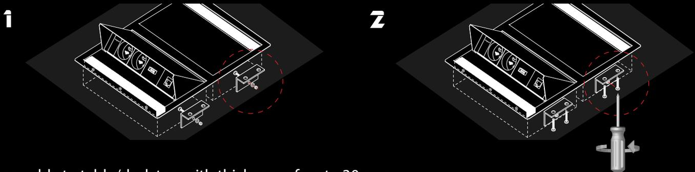
Assembly to table/desk top with thickness of up to 30 mm.
