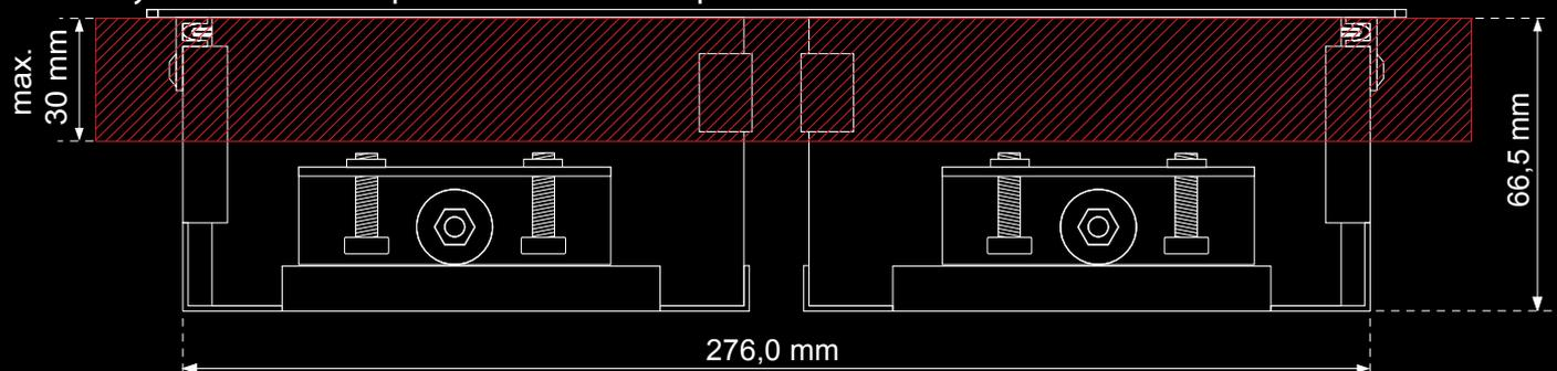
Assembly to table/desk top with thickness of up to 50 mm.
