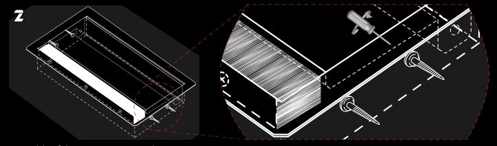
Assembly of the unit using 4 wood screws.
