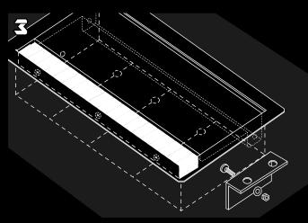
Insert Magnat-Subdesk Multi into mounting hole and assembly of mounting brackets.
