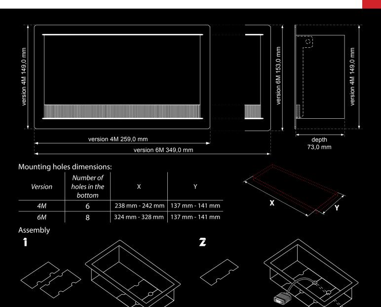
The bottom consists of sections with divided holes which allow to route the cords. These holes protect against pulling out the cords.
